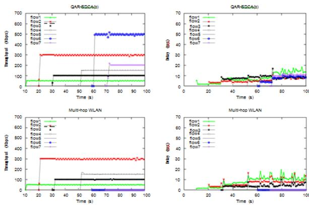
Fig. 7 Instantaneous throughput and instantaneous end-to-end delay over grid topology
