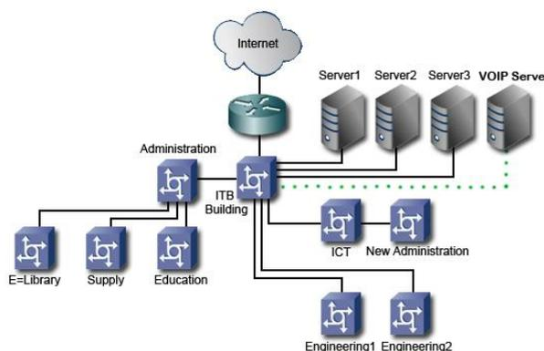
Fig.2. Architectural Design of Networks in MUST with Additional VoIP Server
