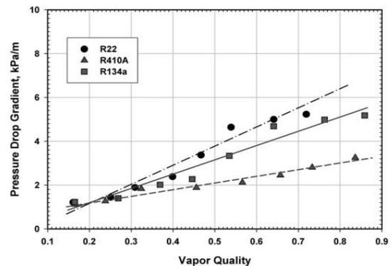
Fig. 6 Comparison of pressure drop gradient at  $G = 100 \text{ kg/m}^2\text{s}$ .
