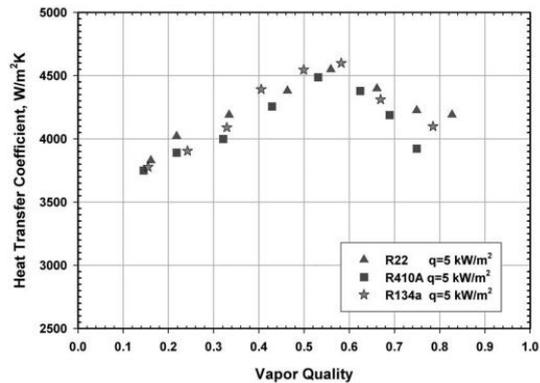
Fig. 5 Comparison of heat transfer coefficients at  $G = 300 \text{ kg/m}^2\text{s}$ .
