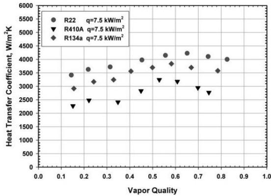
Fig. 4 Comparison of heat transfer coefficients at  $G = 200 \text{ kg/m}^2\text{s}$ .
