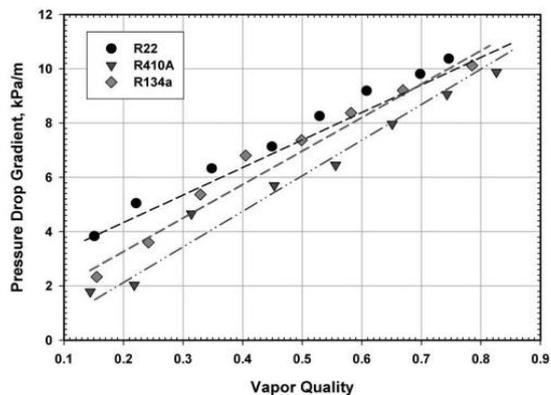
Fig. 7 Comparison of pressure drop gradient at  $G = 300 \text{ kg/m}^2\text{s}$ .
