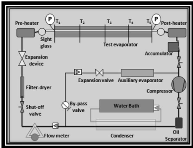
Fig. 2 Schematic diagram of experimental rig.
