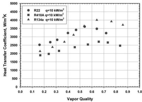
Fig. 3 Heat transfer coefficients comparison at  $G = 100 \text{ kg/m}^2\text{s}$ .
