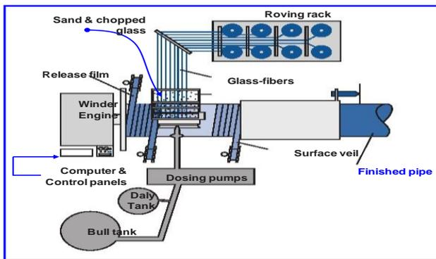
Fig.(1) Schematic Diagram of Continuous Filament winding
