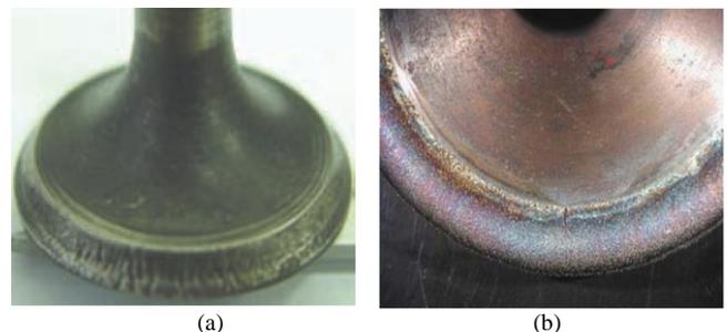
Fig. 2. A view of engine valve face: (a) Erosion wear (22); (b) after LC (23)
