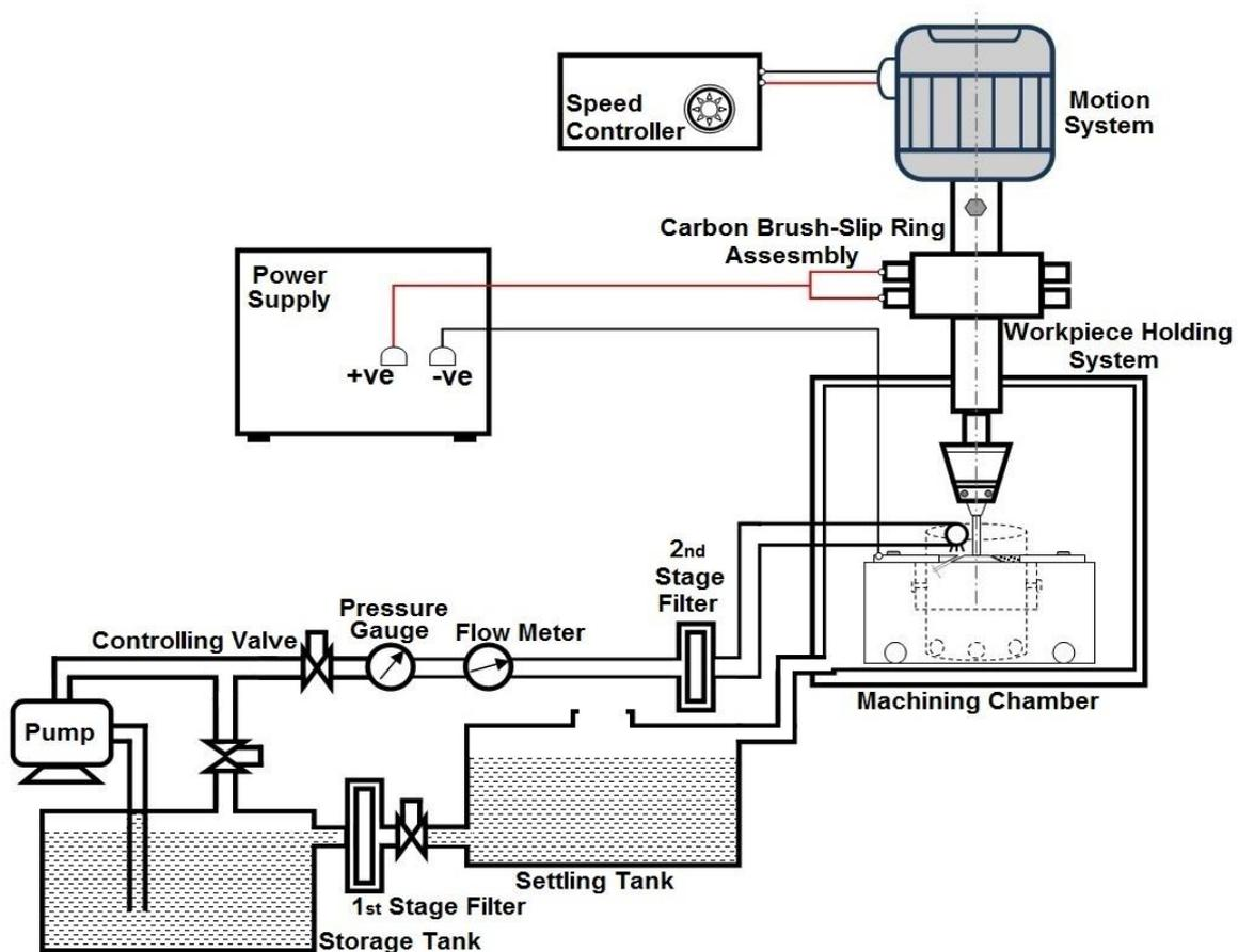
Fig. 3. A schematic diagram of designed experimental setup for remanufacturing of engine valve face through ECH
