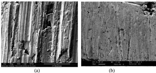
Fig. 1. SEM photograph: (a) before ECH (at 1000x); (b) after ECH (at 1000x) [15]
