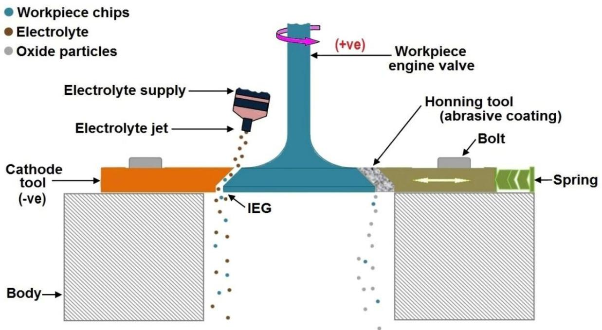
Fig. 5 Proposed process principle of ECH of engine valves
