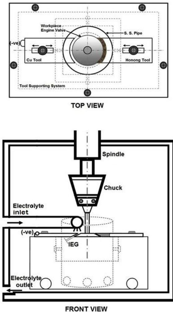
Fig. 4. A schematic diagram of machining chamber with tools and positioning systems in ECH of valve face
