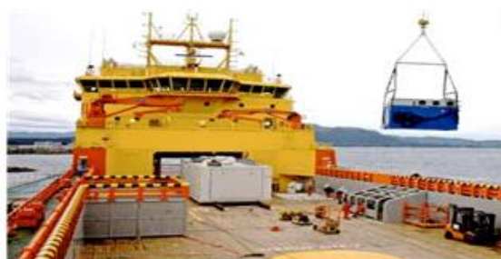
Fig. 1 Fuel Cell Equipment Being Installed On Eidesvik's Viking Lady, Source: Eide And Endresen [12]
