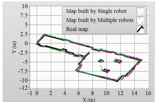
Fig. 6. Comparison of the single and multi-robots mapping accuracy versus real map.
