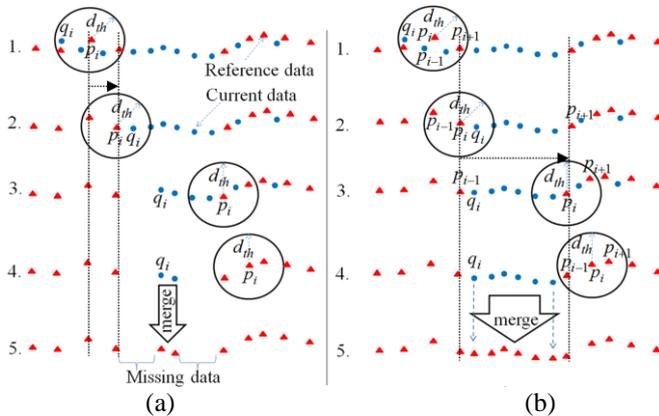
Fig. 2. Map merging. a) Conventional merging rule. b) Modified map merging rule.
