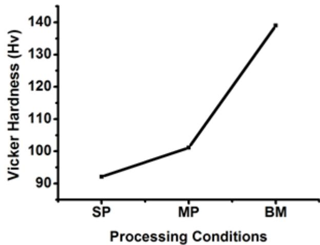
Fig. 6. Plot showing the effect of single pass and multipass friction stir processing on hardness of AA7039.
