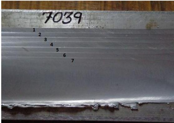
Fig. 2. Photograph of plate subjected to friction stir processing for seven passes.
