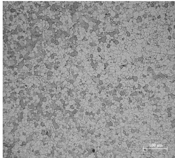
Fig. 4. Optical micrograph of stir zone of friction stir processed AA 7039.
