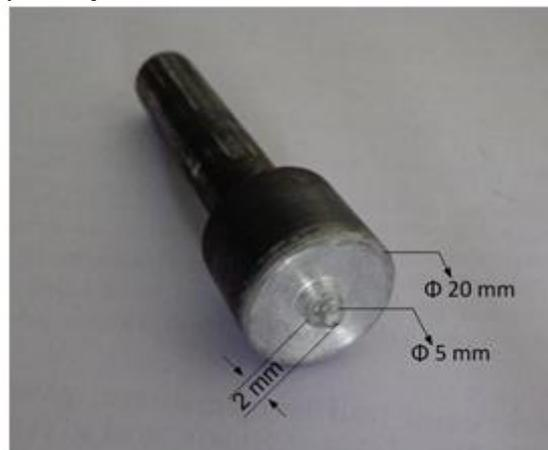
Fig. 1. Photograph of the tool used for friction stir processing.
