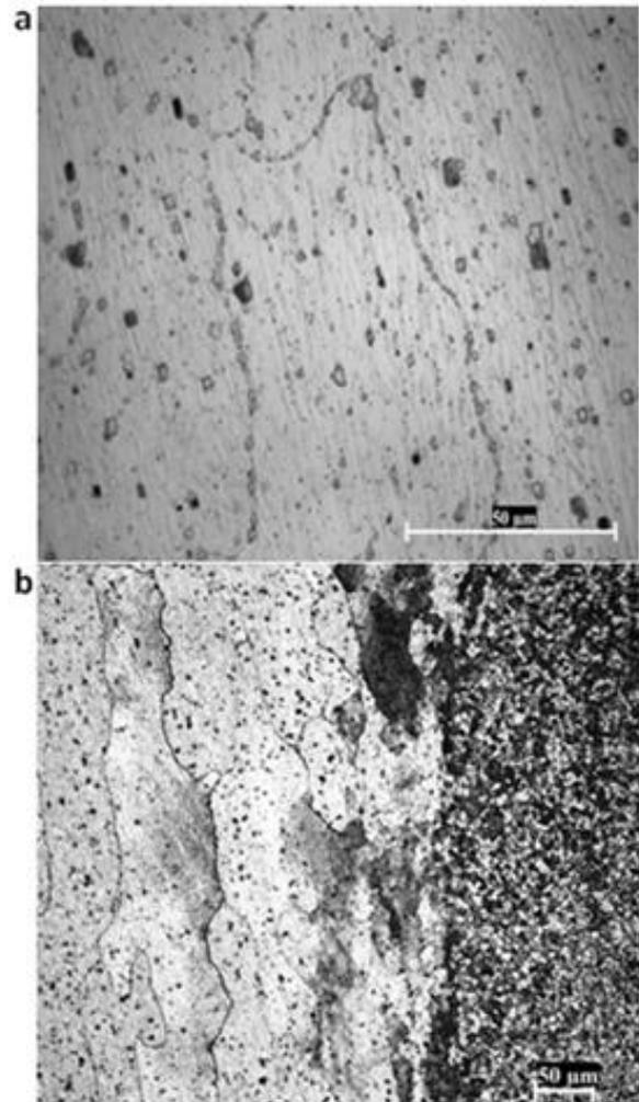
Fig. 3. Optical micrographs of (a) unprocessed AA 7039 alloy, (b) interface of unprocessed and friction stir processed AA 7039.
