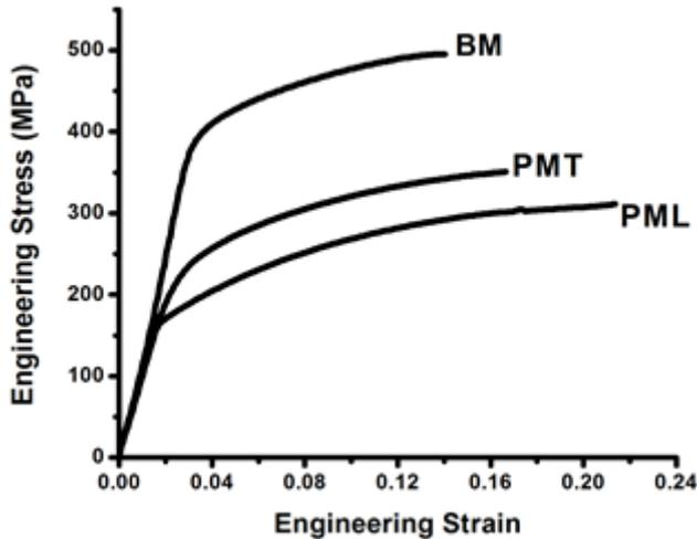
Fig. 5. Engineering stress-strain diagram obtained from tensile test of unprocessed alloy and friction stir processed alloy.
