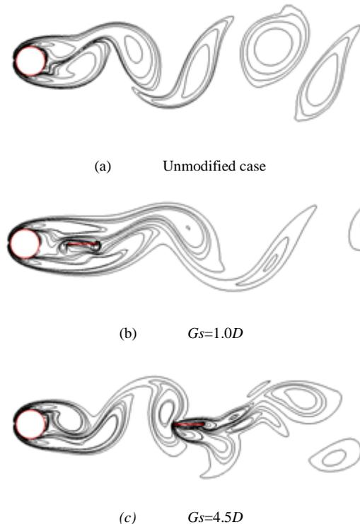
Fig. 5 Transient vorticity contour for the cases with and without a detached plate ( $Re=150, \beta = 0.1, L = D$ )
