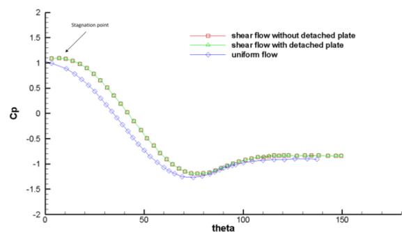
Fig. 2 Comparison of the pressure distributions in uniform flow and shear flow with and without detached plate ( $Re=150$ ,  $\beta = 0.1$ )
