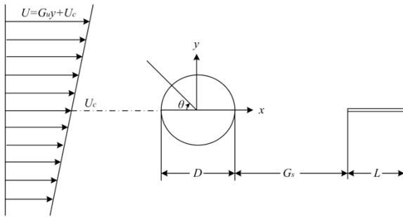
Fig. 1 Model of a cylinder-plate system in a linear shear flow with geometries in a Cartesian coordinate system
