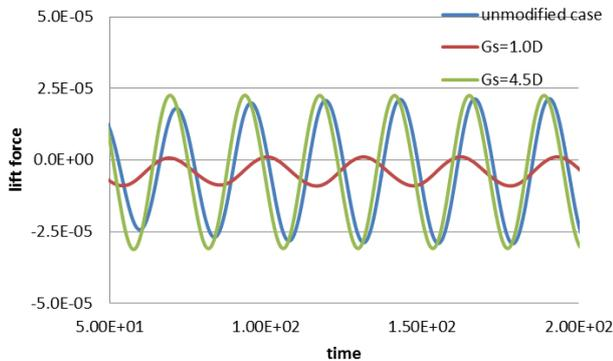
Fig. 3 Stabilization of lift forces with time ( $Re=150, \beta = 0.1, L = D$ ) for the cases with and without detached plate
