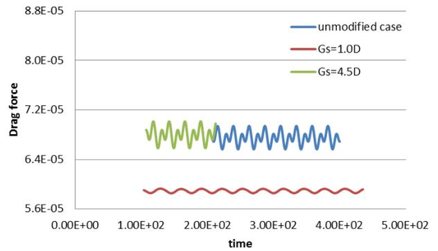
Fig. 4 Stabilization of drag forces with time ( $Re=150, \beta = 0.1, L = D$ ) for the cases with and without detached plate
