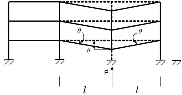
Fig. 1 Beam rotation and joint deflection caused by loss of a column
