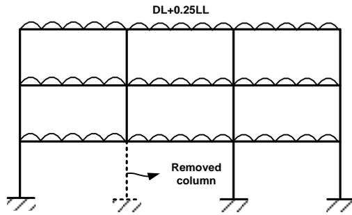
Fig. 3 Imposed load for dynamic analysis
