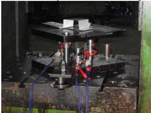
Fig. 5 test apparatus assembled on a press and a tested specimen
