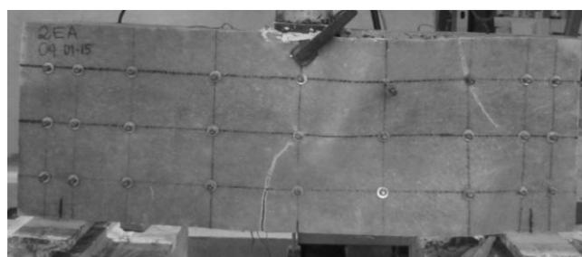
Fig. 9 Failure mode of Beam 2EA.
