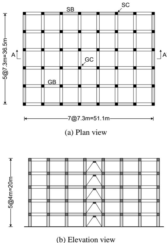
Fig. 2 Configuration of 5-story analysis model structure
