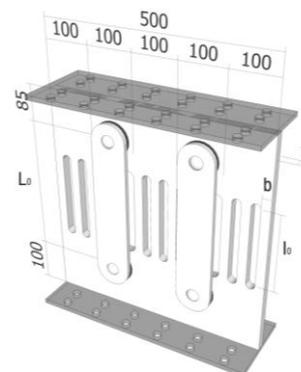
Fig. 1 Configuration of a hybrid slit-friction damper
