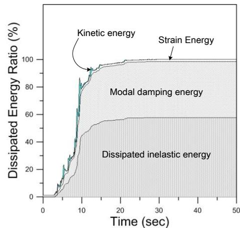
Fig. 6. Energy dissipation in the model structure subjected to Northridge earthquake
